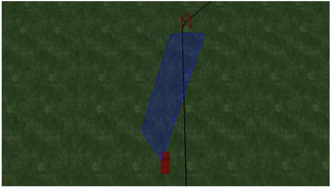
Figure 15. Diagonally-aligned LIDAR sensor configuration (overhead view).
