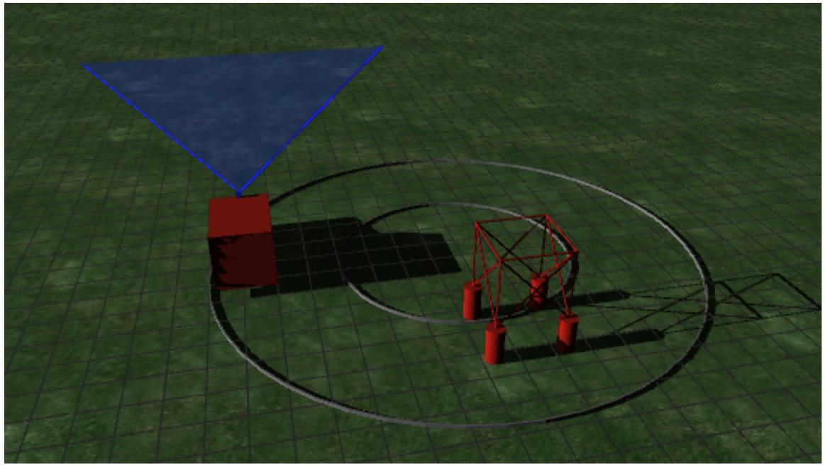
Figure 17. Epsilon Lambda ELSC71-1A RADAR field-of-view limitation (simulation initial state).
